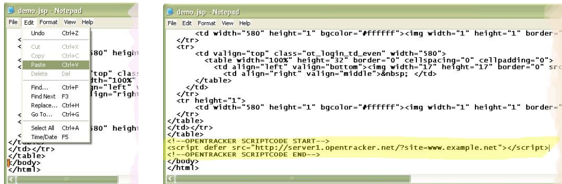
Printscreen of code before pasting (note cursor before </body> tag) and after pasting (code highlighted in yellow to clarify).
